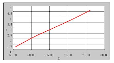
Accordance with the above formula the once in 15 years value of y equal 2.67, the corresponding value of x is 66.4. It means that the standard ice thickness value of once in 15 years on LGJ-400 in the Erlang Mountain Pass zone is 66mm. The design of the ice thickness by height revised can be 76mm.
