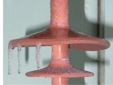
Fig.4 icing experiment of composite insulator
