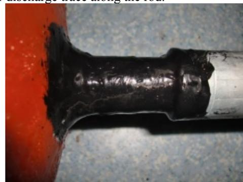
Fig.10 discharge trace along the rod
