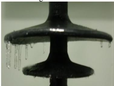
Fig.7 icing experiment of the second sample
