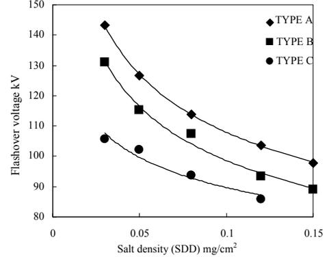
Fig.4  $U_{50}$  versus SDD in Solid-layer method
