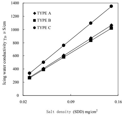
Fig.6 The relation curve between  $SDD_g$  and  $\gamma_{20}$
