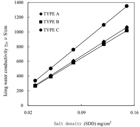
Figure 1. The relation curve between  $SDD_g$  and  $\gamma_{20}$
