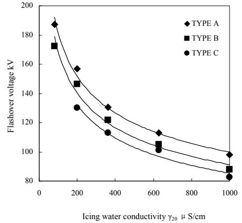
Fig.5  $U_{50}$  versus  $\gamma_{20}$  in icing-water-conductivity method
