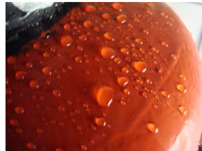
Figure 3: the shape of the water-drop on the surface of the insulator
