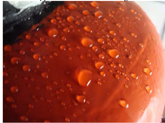
Figure 7 : the shape of the water-drop on the surface of the insulator
