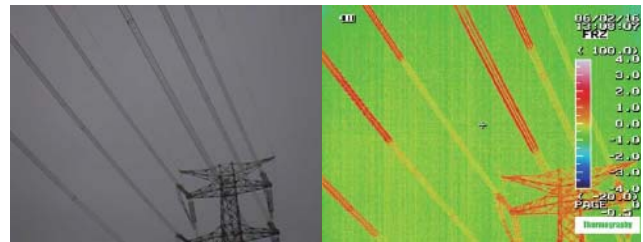
Figure 5. Example of an infrared image (right-hand side) of the actual transmission line (left-hand side) with red parts corresponding to installed sections of LC-Spiral Rods.
