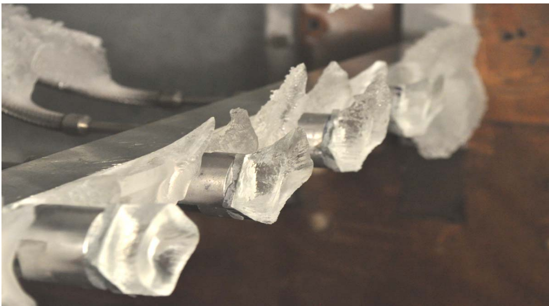
Figure 3: Test rig with secured to icing tunnel and (glaze) ice accreted on coated substrate
