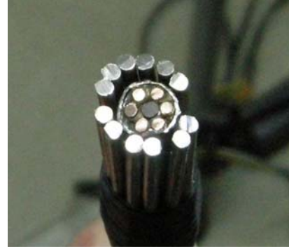
Figure 3. Sample hybrid overhead ground wire.
