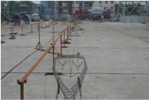
Figure 1. Small-scaled Simulated Compact Transmission Line
