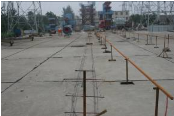
Figure 2. Small-scaled Simulated Double-circuit Transmission Line
