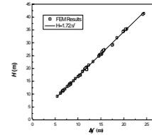
Fig.7 Relation between jump height and sag difference of electric line before and after ice-shedding
