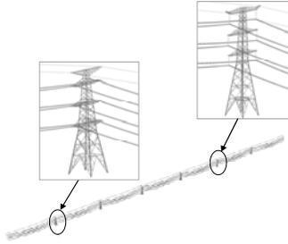
Fig. 2: Finite element model of the typical transmission tower-line system with seven spans
