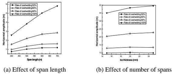
Fig. 6 Effect of different factors on horizontal swing amplitude
