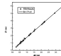
**Fig.8** Relation between horizontal swing amplitude and swing difference of electric line before and after ice-shedding
