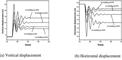
Fig. 3 Dynamic displacements of mid-point of conductor line after ice-shedding
