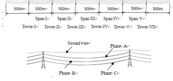
Fig. 1: Transmission tower-line section with seven spans
