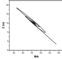
Fig. 4: Moving trace of mid-point of a conductor after ice-shedding
