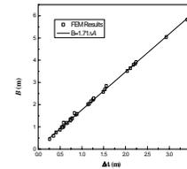
**Figure2:** Relation between horizontal swing amplitude and swing difference of electric line before and after ice-shedding
