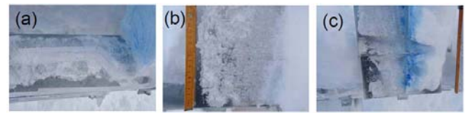
Figure 9. Examples of conditions of surfaces after removing snow on (a) cross beam without countermeasure, (b) tilted flat plate, (c) tilted stepped plate observed in the first observation.
